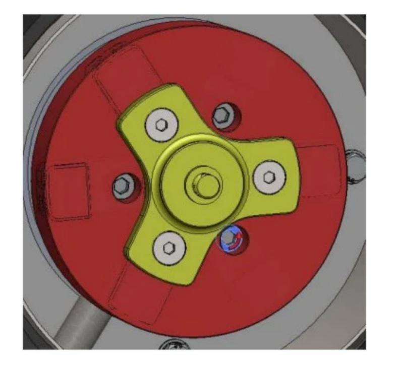
MET-25228 Red Cast Urethane Coupling (2008 - 2015) This non serviceable coupling was also cast in black.
