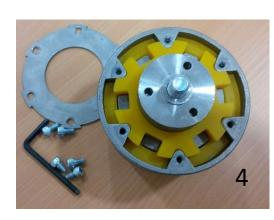
**To Change:** Remove the six socket head cap screws, cover plate, and the first yellow polyurethane element only (1). Now re-install the first element, with the element turned  $30^{\circ}$  so the V sections engage the perimeter V drives on the stainless steel coupling body (4). Re-assemble the coupling. The coupling is now on 'Soft' setting (4).
