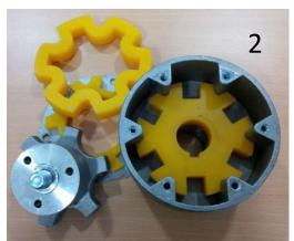
yellow polyurethane elements (1). Insert the three new elements. The first has the keyway in the centre hole (2), ensure the V sections engage the perimeter V drives on the stainless steel coupling body. The second element slides down the six perimeter V drives (1). Insert the Stainless Steel Disc Mount with M14 Thread (1). Push in the last element, please note correct
