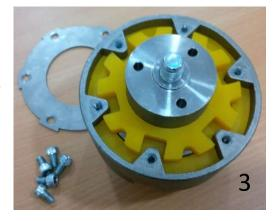
Hard Setting: Use the 'Hard' setting when the Meteor 250 is to be used extensively for trip hazard removal. The coupling can be set to 'Hard' by turning the back element 30°, as well as the front element being set as 'Hard' (3).
