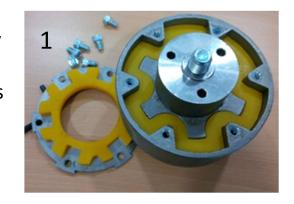
position (3), fit the Stainless Steel Cover plate, and then tighten the six socket head cap screws tightly. The use of thread locker on the cap screws is recommended.
